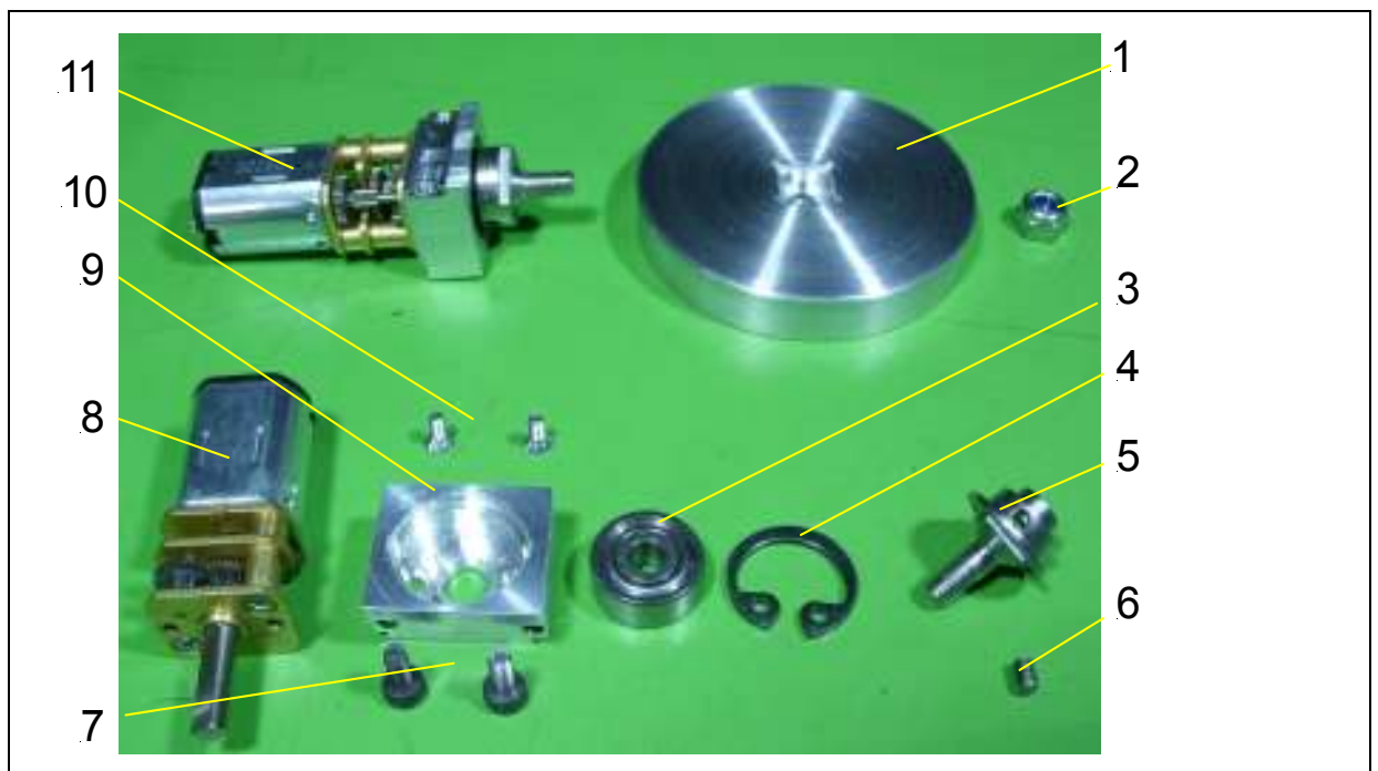
Fig. 5: Montage material for DC motor
