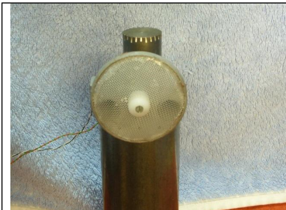
Fig. 7a: Small Longhorn, - Ear distance 30 mm, - With a thin mesh provided by a sieve for milk
