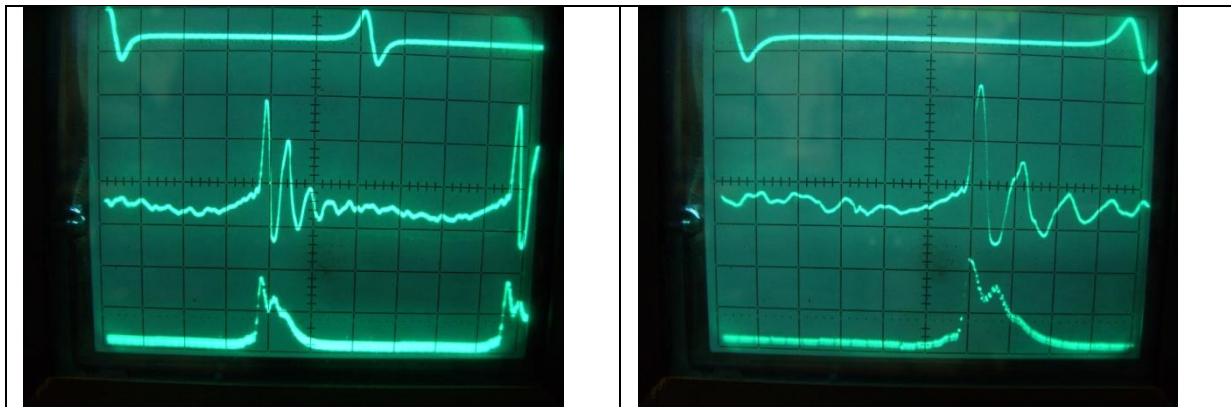
Fig. 3c: Motor Supply 4V, 100ms/Div Max Current: 380mA Average Current: 50mA Stroke force: 1.25N
