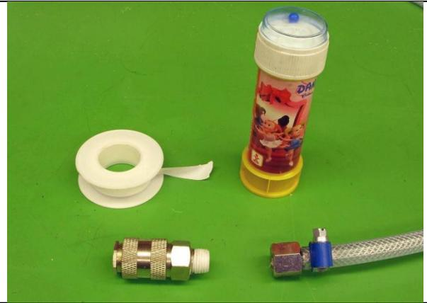
Fig. 10: Pneumatic tube assembly and leakage test by soap water. Teflon tape on threads. A small leakage was detected by soap water!
