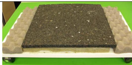
Fig. 7: Bottom plate with mineral wood and shock absorber plate above
