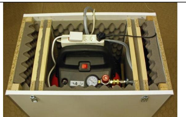
Fig. 14: Installed pin strip with flat 230V plugs
