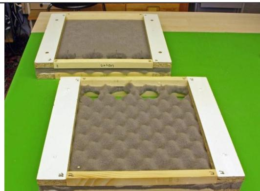
Fig. 5: Air guide frames, with pinched foam rubber and holes of 50 mm diameter
