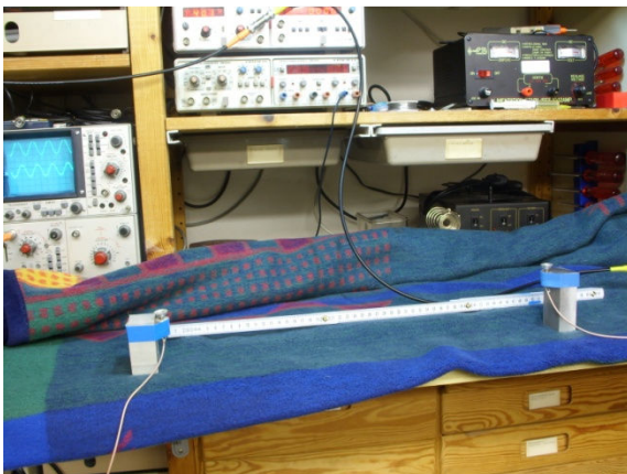
Fig. 5. Transmitter and Receiver upwards with Radial Radiators: Received: 4mVpp
