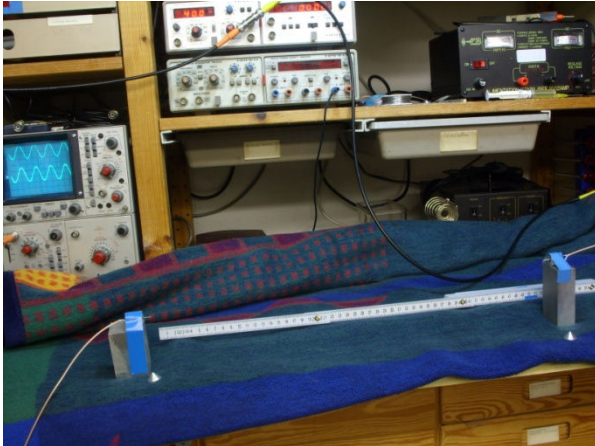
Fig. 3. Standard , transmitter and receiver axial face to face : Received: 125mVpp
