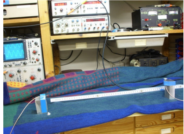
Fig. 4. Transmitter upwards with Radial Radiator, receiver standard axial: Received: 35mVpp
