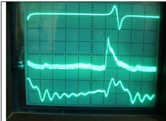
Fig. 4b: Motor Supply 5V Max Current: 165mA Max Stroke force: 0.6V, 0.34N
