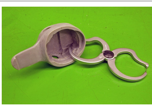
Fig. 16: Check always wall thickness!
