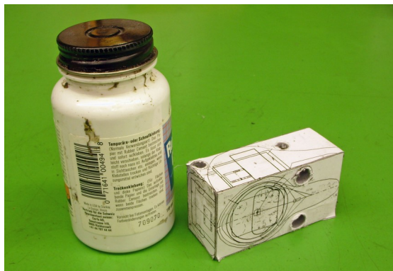
Fig. 11: Template glued on PVC block
